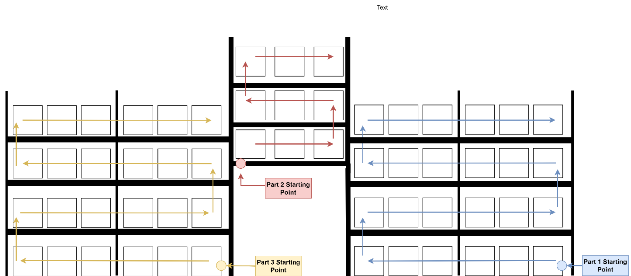
FIGURE 2-6 - RECORDING AISLE WITH MISALIGNED SHELVES ON THRU/ARCH
